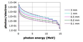
Figure 4: Bremsstrahlung spectra of a 15-MeV electron beam hitting tungsten targets of different thicknesses.
