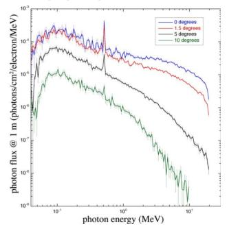
Figure 5: Bremsstrahlung spectra at different angles after traversing a 30-cm aluminum. The bremsstrahlung is produced by a 20-MeV electron beam hitting a 0.1 mm tungsten target.
