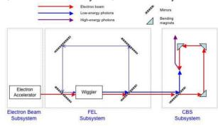
Figure 2: Schematic of a CBS Source
