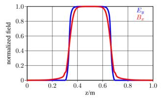
Figure 3: Normalized electric and magnetic field of Wien filter.
