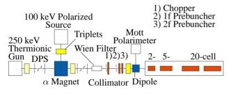
Figure 1: Sketch of the S-DALINAC injector in the accelerator hall.
