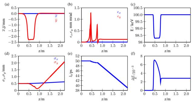
Figure 5: Transverse and longitudinal beam dynamics results through the Wien filter.
