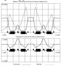
Fig. 5: Low vertical beta-optics in the long straight sections of ANKA:  $\beta_x = 14 \text{ m}$ ,  $\beta_v = 1.9 \text{ m}$ ,  $\varepsilon_x = 40 \text{ nm}$
