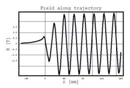
Fig. 3: Field of the superconducting wiggler shown in Fig. 2. The period length is 21 mm, the gap is 5 mm, the current  $1 \text{ kA/mm}^2$  and K = 5.26
