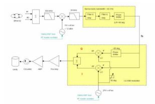
Figure 2: Block diagram of anlog mode feedback system. A high power circulator was not installed during this experiment.
