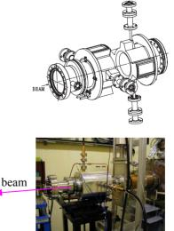
Figure 1: Drawing and a photo of the longitudinal kicker installed at downstream of the RF accelerating cavity. Blue cables in the photo are temperature sensors.
