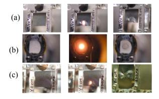
Figure.6 Photographs of (a)a double-layered HBC-foil, (b)a DM-foil and (c) a CM-foil at different stages of irradiation.
