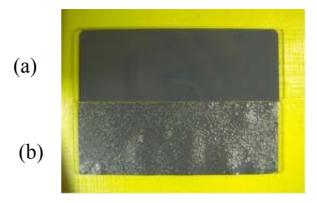
Figure.4 Photographs of carbon layers on slide glasses. Represent an HBC-foil of 370  $\mu$ g/cm<sup>2</sup> and is for a Cluster–foil of 140  $\mu$ g/cm<sup>2</sup> made by the CADAD method.
