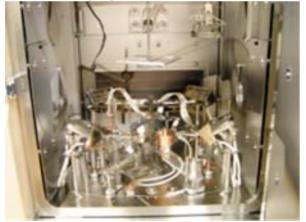
Figure.3 Arc-discharhe evaporation-source in EBX-2000C cryo-vacuum pump apparatus.
