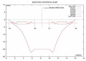
Figure 1: SESAME injection horizontal bump scheme.
