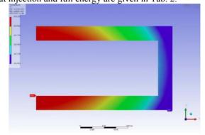
Figure 5: Temperature distribution for 1µm titanium layer thickness.
