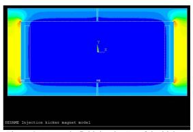
Figure 2: Magnetic field density By of the kicker.
