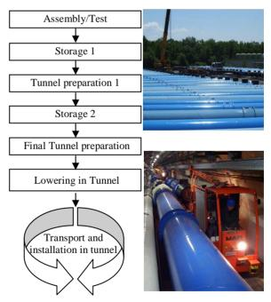
Figure 2: The logistics chain of a LHC cryo-magnet.
