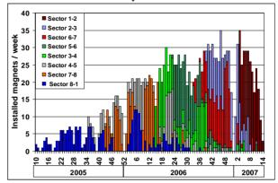
Figure 3: The LHC cryo-magnet installation rate.
