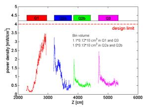
Figure 2: Longitudinal distribution of the peak deposition in the first layer coil. IR1 vertical crossing plane, FDDF magnets,  $L=10^{34}$  cm<sup>-2</sup>s<sup>-1</sup>.
