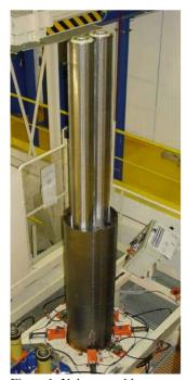
Figure 1: Yoke assembly around quadrupole apertures
