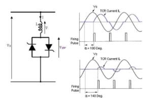
Fig. 1. TCR Configuration and Operation
