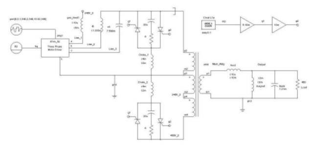
Fig. 2. Saber Schematic for the ISIS White Circuit with Static VAr Power Factor Correction
