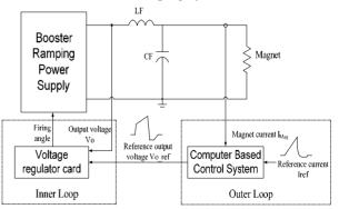
Figure 2: The block diagram of the voltage-mode controlled ramping power supply.
