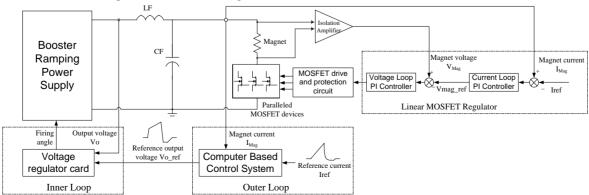
Figure 3: Block diagram of the proposed MOSFET linear regulation system for the ramping power supply.
