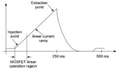
Figure 1: A typical magnet current ramp cycle in the booster.
