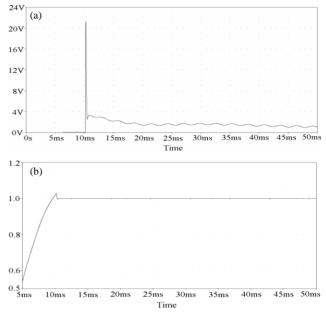
Figure 5 (a): Voltage drop on MOSFET devices during the MOSFET linear operation region during the MOSFET linear operation region, (b): around the injection point.
