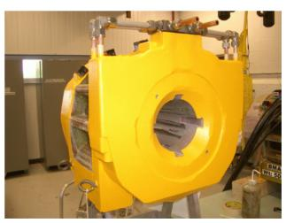
Figure 2 Corrector without BPM after potting and painting.
