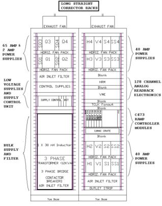
Figure 3 Layout of Long Straight Corrector Racks
