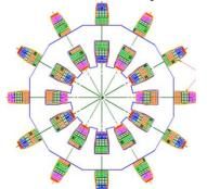
Figure 2: Coil arrangement in new correctors
