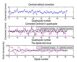
Figure 3: Beam centroid correction with earth field. In the upper figure, we assume there is a random error in the quadrupole center. The center figure shows the corrected beam centroid with conventional control and the calibrated control. The bottom figure shows the bending force required in each dipole.
