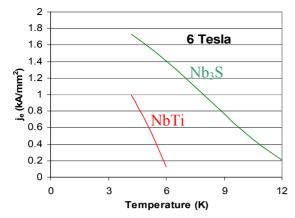
Figure 5:  $j_E vs$ . T for NbTi and N<sub>3</sub>Sn.
