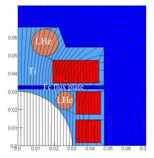
Figure 3: Structural design of rapid-cycling dipole.
