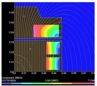
Figure 2: Field distribution in rapid-cycling block-coil dipole.  $B_{mod}$  is shown in coil blocks.
