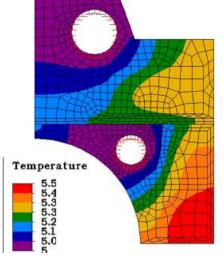
Figure 6: Temperature profile with supercritical cooling; the coil is dissipating 48 W/m at 9 T/s ramp rate.
