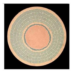
Figure 4: Cross-section micrograph of Furukawa bronze-process  $Nb_3Sn$  strand: 9800 filaments, 0.8 mm diameter.
