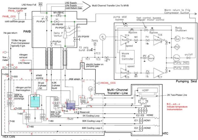
Figure 1: Cornell ERL injector cryogenic system diagram.
