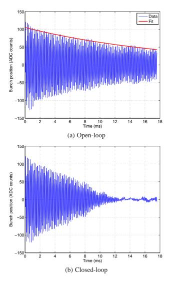
Figure 2: Single-bunch longitudinal motion immediately after injection
