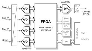
Figure 3: Signal channel hook-up of the digital hardware for the ring rf control application.
