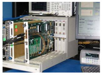
Figure 4: The first prototype of SNS digital ring rf control under bench test.
