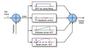
Figure 2: The combined feedback and feed forward control scheme for the ring rf offers a better capability in handling the heavy beam loading and the flexibility for the study of various control methods.
