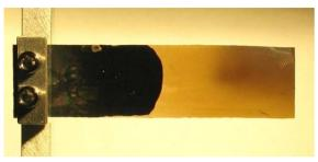
Figure 3: SNS 12x20 mm<sup>2</sup> foil after use. The image has been rotated 90° CCW from the true orientation. Damage is apparent in the figure upper right corner.
