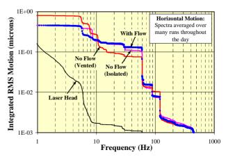
Figure 4: Integrated spectra with and without helium flow, averaged over all runs during the day.
