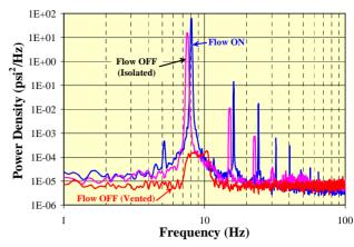
Figure 7: Power density spectra of helium pressure variations in the magnet with and without flow.
