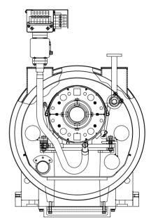
Figure 1: Cross section of a RHIC quadrupole cold mass in its cryostat.
