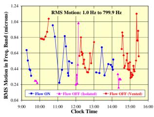
Figure 5: Cold mass RMS motion above 1 Hz.
