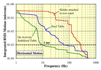
Figure 3: Laser holder motion in the earlier setup, and in the new setup with and without stabilization. The curves give the total RMS motion at or above any given frequency. Steps in the curves correspond to prominent peaks in the power spectrum.
