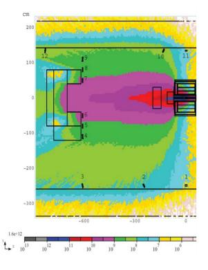
Figure 5: Secondary pion fluxes for a pulse of  $3 \times 10^{13}$  24-GeV protons on an Hg target, shown in the horizontal plane at beam height, according to the MARS code. The positions of 12 particle detectors are indicated in the figure.
