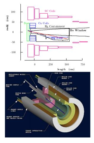
Figure 1: Concept of a continuous mercury jet target for an intense proton beam. The jet and beam are tilted by 100 mrad and 67 mrad, respectively, with respect to a 20-T solenoid magnet that conducts low-momentum pions into a decay channel.
