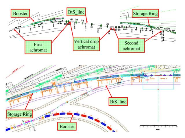
Figure 1: Drawing of the two proposed BtS transfer lines. In the top drawing, Booster and SR share the same tunnel. The three line-sections of the BtS line described in the text are labeled and their extend is indicated by red arrows. In the bottom drawing Booster and SR are in separate buildings.
