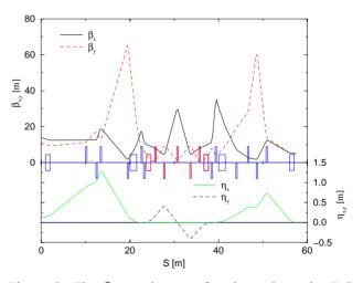
Figure 2: The  $\beta_{xy}$  and  $\eta_{xy}$  functions along the BtS transport line. The "blue" and "red" wide rectangular boxes are the dipoles and thin ones are the quadrupoles used in the transport line respectively. The magnetic elements of "Vertical drop achromat" line-section are the "red" rectangular boxes.
