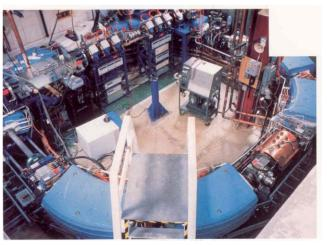
Figure 2: LLUMC weak focusing 250 MeV synchrotron.
