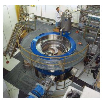
Figure 1: COMET superconducting isochronous cyclotron (partially disassembled).
