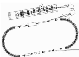
Figure 3: RCMS Rapid Cycling Medical Synchrotron.
