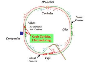
Figure 2: The layout of the crab cavities at KEKB with the LER (red) and the HER (green). Each ring has one crab cavity at the Nikko straight section where the cryogenics already exists for the accelerating cavities. Each ring is equipped with a streak camera.
