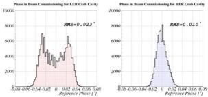
Figure 4: Phase distribution of the crab cavities for the LER (left) and the HER (right) with the rf feedback. The standard deviations of the phases are 0.023 deg and 0.010 deg for the LER and the HER, respectively.
