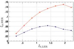
Figure 1: Enhancement of the vertical beam-beam parameter by a head-on (crab) collision (upper curve) comparing to the crossing angle of 22 mrad (lower curve), obtained by a strong-strong beam-beam simulation. Parameters are same as the present KEKB.
