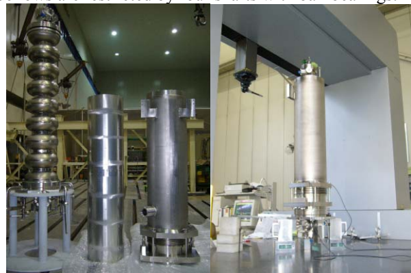
Figure 6: Before and after welding of a helium jacket. A magnetic shield (centre in left) was inside of a helium jacket.
