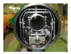
Figure 6: Cross section of the cryostat being assembled.
