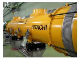
Figure 7: STF cryomodule as completed.
