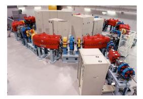
Figure 5: Multi-purpose accelerator with synchrotron and tandem.
