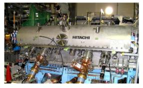
Figure 3: RFQ as installed.
