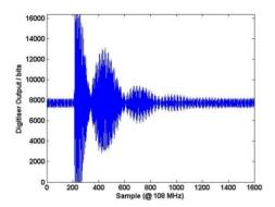
Figure 2: Example of the output of the HOM electronics for a single bunch beam.
