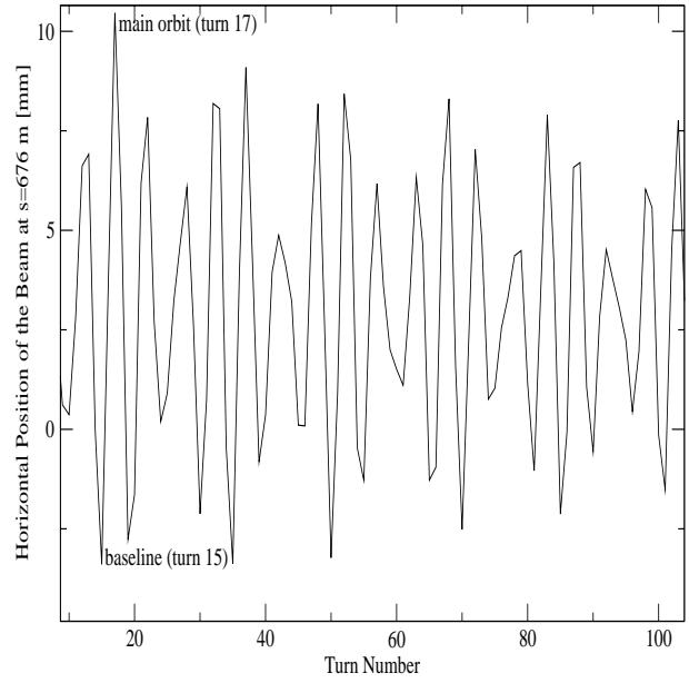
Figure 4: This plot helps to choose appropriate turns to build a difference orbit. For the example of this section, turns 17 and 15 are chosen due to their amplitudes.
