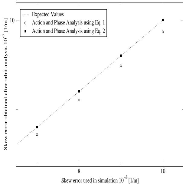
Figure 1: Relation between the skew quadrupole errors used to simulate RHIC orbits and the skew quadrupole errors recovered using action and phase analysis on the simulated orbits. Differences between previous (circles) and current (squares) simulations are shown.
