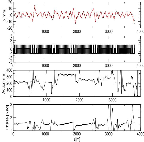
Figure 3: Action and phase jump analysis of a RHIC difference orbit. This time the difference is built from turns 17 and 15 of the same orbit bi8-qs3.-0.0010.8h.sdds.
