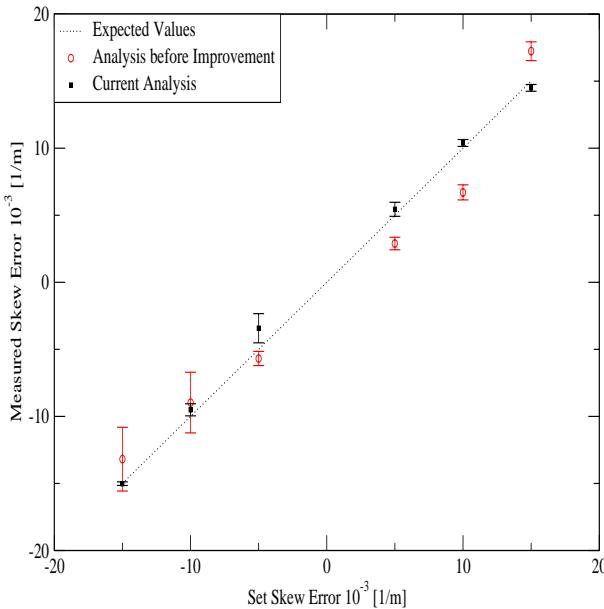
Figure 5: Skew quadrupole errors recovered using the conventional (red circles) and the new (black squares) action and phase analysis on experimental orbits.
