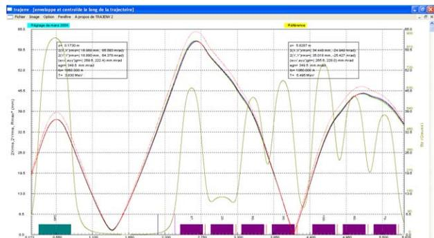
Figure 5: Beam envelope given by the TRAJENV code.
