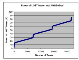
Figure 2: Power of the lost beam of the 2kW/bunch beam power at the MR collimator with the physical acceptance of 54  $\pi$  mm.mrad and for the 'bare' working point  $Q_x=22.30$ ,  $Q_y=20.92$  during the 'full-time' injection
