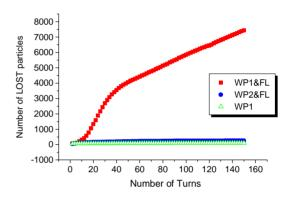
Figure 1: Particle losses as a function of turn number for different 'bare' working points in the case of the field leakage of the opposite field septum.
