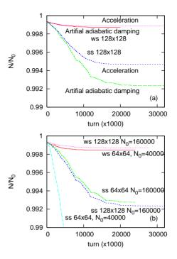
Figure 2: Beam loss for the collimator aperture  $70\pi$  mm·mrad.
