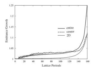
Figure 3: Evolution of the rms emittance during the beam transport with the pulse compression. The solid curve indicates the emittance growth over the entire beam bunch, the dashed line shows one evaluated near center of the beam bunch, and the dotted line shows for the 2D sliced calculation result with the longitudinal compression model.
