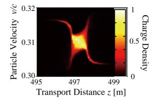
Figure 4: Normalized charge distribution in the longitudinal phase space at the stagnation point.
