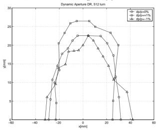
Figure 5: Dynamic aperture (DA) for high alpha case, with all magnets errors and misalignment errors.
