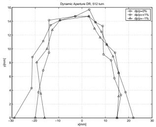
Figure 6: Dynamic aperture for low alpha case, with all magnets errors.
