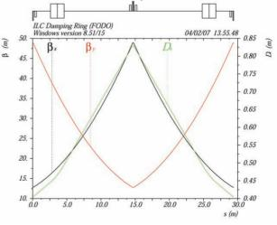
Figure 1: Lattice functions in an arc cell.
