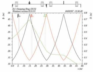
Figure 2: Lattice functions in a dispersion suppressor.
