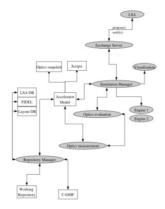
Figure 1: Software Architecture Design
