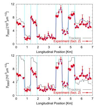
Figure 3: Longitudinal Driving Term Pattern due to one failing Sextupole.
