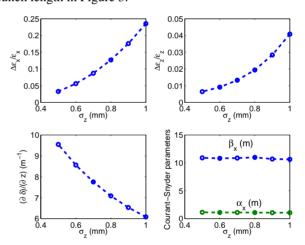
Figure 2: Transverse and longitudinal emittance errors along with optimum chirp and Courant-Snyder parameters as functions of the incoming bunch length. The incoming beam emittance was  $(\varepsilon_{x,0},\varepsilon_{z,0})=(10,3)~\mu\mathrm{m}$ .
