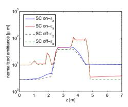
Figure 6: Emittance evolution along the emittance exchanger beamline, with and without consideration of space-charge effects.
