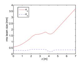
Figure 5: Beam size evolution along the emittance exchanger beamline.
