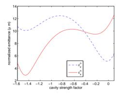
Figure 4: Beam longitudinal and transverse emittance as functions of the dipole mode cavity strength.
