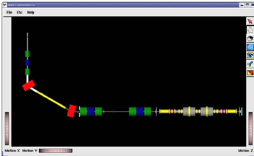
Figure 2: The MICE muon beamline and cooling channel [3] – a detailed and realistic simulation using G4beamline. Quadrupoles are green (HF) and blue (HD), dipoles are red, solenoids are yellow, beam pipes are gray, vacuum chambers are white, the two RF cavities are gray, and the calorimeter at the end is light blue. The pion production target is at the top left inside the ISIS synchrotron (not shown).
