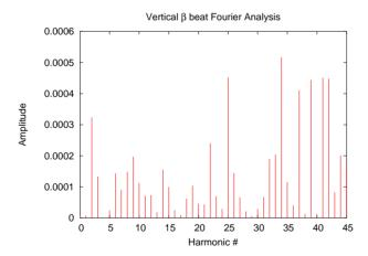
Figure 4: Vertical  $\beta$ -beating Fourier spectrum.
