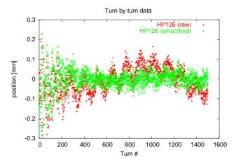
Figure 8: Horizontal TBT for a  $N=1.5\times10^{12}$  case.
