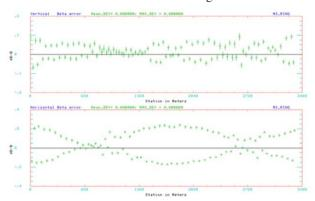
Figure 7. Beta error at 150 GeV. Maximum vertical error is below 10% and maximum horizontal error is over 25%, bottom plot with its vertical scale range doubled, to ±0.4 from ±0.2.
