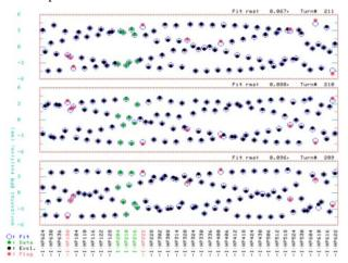
Figure 1. Example of horizontal plane TBT data, ring-wide and for 3 consecutive turns, from 8-GeV measurement.
