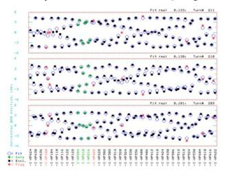
Figure 9. Horizontal plane TBT data from 150 GeV measurement. Agreements between projections and data are visibly poor. This is a complimentary view of what was shown in Figure 8.
