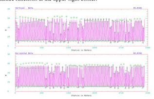
Figure 4. Measured Main Injector 8-GeV beta function. Bottom plot is for horizontal plane and top plot vertical plane. Green circles are measured beta functions and magenta traces are the design values. Statistical beta errors are plotted as vertical lines, i.e. the barely visible short vertical lines inside the circles.
