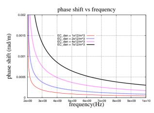
Figure 2: Plots of phase shift per unit length for different electron densities with  $\omega_c = 2$ GHz.
