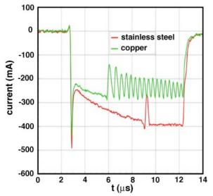
Figure 1: Current through 50  $\Omega$  to ground from a positively biased deflector plate using a stainless-steel target plate (red) and a copper one (green). A 5-kV bias was used here, and similar results were found for higher voltages.
