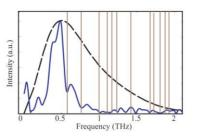
Figure 4: The dashed curve is the QUINDI results. The solid curve is the experimental data from BNL. The vertical lines are water absorption lines, corresponding to local minima in the data.[1]
