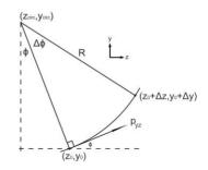
Figure 2: Geometry used for calculating position and momentum.
