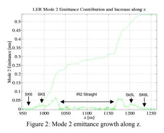
Skew quadrupoles SK5 and SK6 on each side were originally used in a symmetric fashion to generate the necessary coupling to cancel the coupling from detector solenoid field, but keeping the vertical dispersion small. However, this creates a significant emittance growth due to coupling. To reduce this effect additional skew quadrupoles have to be added in the IR2 straight and the strength of SK5 and 6 reduced to zero.
