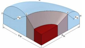
Figure 2: Quarter model of cathode with first and second parts of focus electrode.
