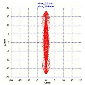
Figure 4: Example for another gun design: a beam cross section in the middle of tuning process is shown. Here the different electrons undergo different focusing and there is a strong aberration effect.
