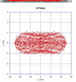
Figure 3: Result of 250 kV, 94 A sheet beam gun design: a), b) top and side views, c) beam cross section near crossover in the tunnel, and d) zoom up beam cross section.
