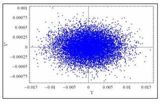
Figure 4. ILC DR bunch at injection as input for simulations, y y' phase space is shown.
