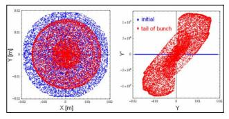
Figure 3. Pinching effect. (Left) x-y and (Right) y-y' phase spaces, cloud distribution at the head (blue dots) and tail (red dots) of bunch pass. The initial cloud distribution is uniform and cold.
