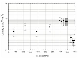
Figure 2: Density measurements along the axis of the BaTiO<sub>3</sub> FEPS indicate that the five sources are balanced in the mid-10<sup>10</sup> cm<sup>-3</sup> density range.
