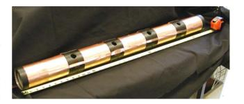
Figure 1: The one-meter-long BaTiO<sub>3</sub> FEPS consists of five individual sources with diagnostic ports between the sources.
