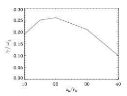
Figure 2: Growth rate  $\gamma$  as a function of bunch aspect ratio  $z_b/r_b$  for high-intensity anisotropic charge bunchs.
