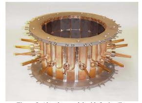
Figure 5: Absorber model with ferrite tiles
