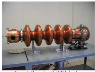
Figure 1: Cu cavity with HOM absorber
