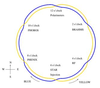
Figure 1: Schematic view of the Relativistic Heavy Ion Collider with its two superconducting storage rings "Blue" and "Yellow," intersecting at six locations around the ring circumference.
