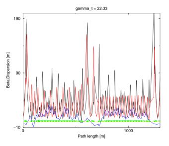
Figure 7: Lattice with transition lowered using the transition jump quadrupoles,  $\Delta \gamma_t = -1.0$ .
