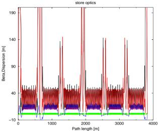
Figure 4: Store lattice with the horizontal tune lowered by one unit. Three interaction regions are squeezed to low  $\beta$  for experiments STAR, PHENIX, and the polarimeter.
