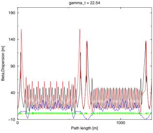
Figure 8: Optics of the hybrid solution, with  $\Delta \gamma_t = -0.8$ .
