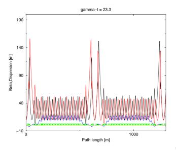
Figure 2: Baseline optics of one third of the RHIC ring, comprised of an inner and an outer arc.
