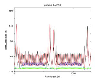
Figure 3: Injection lattice (one superperiod) with the horizontal tune lowered by one unit.
