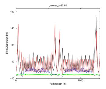
Figure 6: Lattice with transition lowered using the transition jump quadrupoles,  $\Delta \gamma_t = -0.5$ .
