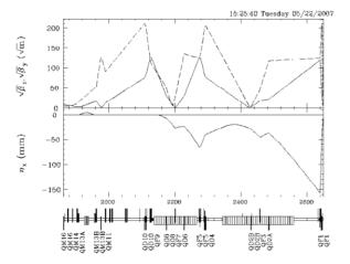
Figure 7: Optics with PMQ. top: original, bottom: using PMQ with partial optimization.
