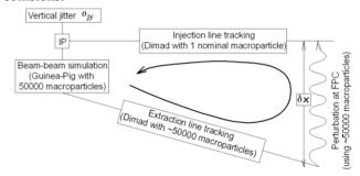
Figure 3: Scheme of the simulation loop.
