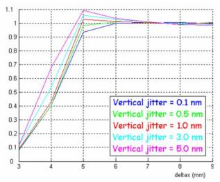
Figure 4: Relative luminosity (L0/L<sub>with KINK</sub>), for a "Guinea-Pig + DIMAD 50000 macro-particles" modelling versus distance between bunches at the FPC (Nominal parameter at 500 GeV center of mass).
