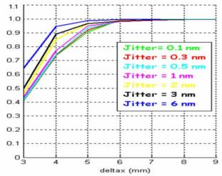
Figure 5: Relative luminosity ( $L0/L_{with\ KINK}$ ), for a "one macro-particle" modelling versus distance between bunches at the FPC (Nominal parameter at 500 GeV center of mass).
